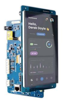
**5-inch to 32-inch** high-resolution, high-brightness displays with flexible options for customization available
